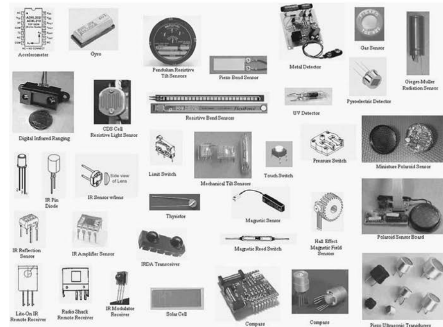
Figure 1.3. Types of sensors. Sensors detect and measure stimuli through a wide range of inputs, including chemical, mechanical, and biological sources. The sensor assemblage typically involves using electronics and software to convert stimuli into electrical and digital signals. Screen capture.
